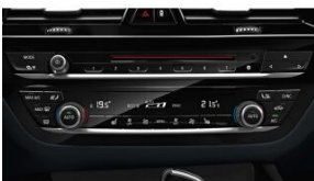
AUTOMATIC AIR CONDITIONING 534
